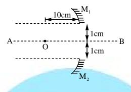
41. Two concave mirrors each of radius of curvature 40 cm are placed such that their principal axes are parallel to each other & at a distance of 1cm to each other. Both the mirrors are at a distance of 100 cm to each other. Consider first reflection at  $M_1$  and then at  $M_2$ , find the coordinates of the image thus formed. Take location of object as the origin.
